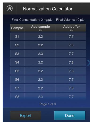
**Figure 8. Normalization Calculator.** The Normalization Calculator quickly provides the amount of sample and buffer needed to normalize to a final concentration and volume. It can easily be transferred via Wi-Fi, USB, or directly to a computer via USB cable.
