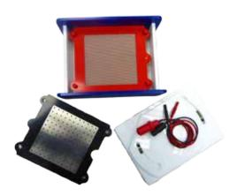
The BlueBlot Semi-Dry Blotter consists of a spring-mounted anode and a drill holes carrying cathode made from stainless steel. The housing is closed with the lid and secured by a newly developed rotating device mechanism. Due to the design of the cable pins wrong connection is excluded.
