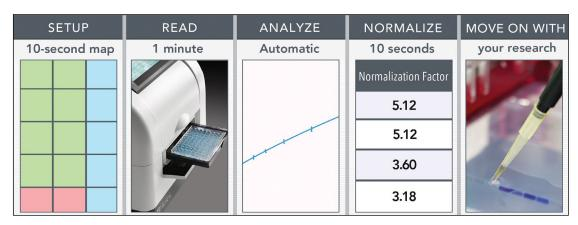
The Quantitative Assay Apps use the power of Gen5 behind a simple, step-by-step customization of predefined protocols for a streamlined process. Bradford, Lowry, BCA or Fluorescence DNA assays are run with only a few clicks.
