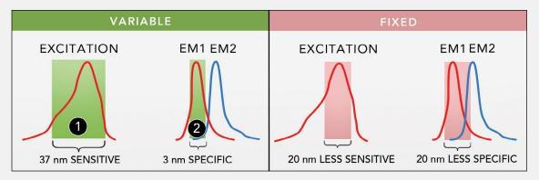
BioTek's Synergy<sup>™</sup> Neo2, Synergy H1 and Cytation C10/7/5 have variable bandwidth monochromators. Large bandwidth settings (1) provide increased sensitivity and lower limits of detection. Small bandwidth settings (2) provide increased specificity when multiple signals are present, which reduces signal crosstalk and enhances assay performance.
