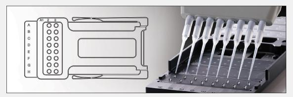
Your BioTek Cytation or Synergy reader becomes a micro-volume analysis system with the Take3<sup>TM</sup> plate. Measure 16 or 48 samples in one run, saving a lot of time compared to single-sample devices. Gen5<sup>TM</sup> is pre-programmed for ssDNA, dsDNA, RNA and protein quantification in 2  $\mu$ L samples.
