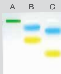
Figure 4. Reaction mixture with DreamTaq Green Buffer (A) prior to electrophoresis, (B) 5 min after electrophoresis, and (C) 15 min after electrophoresis.
