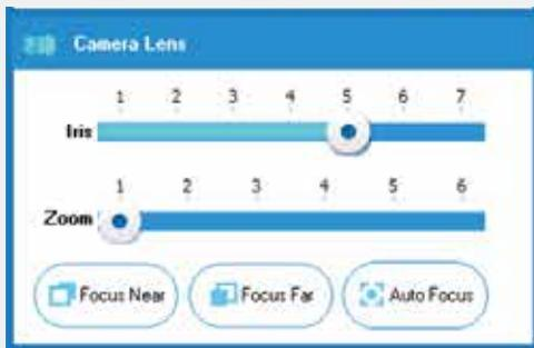
As shown on the left, the aperture size and focus length can be adjusted by pulling the slider. To click the corresponding icon to enter focal fine adjustment or auto focus function.
