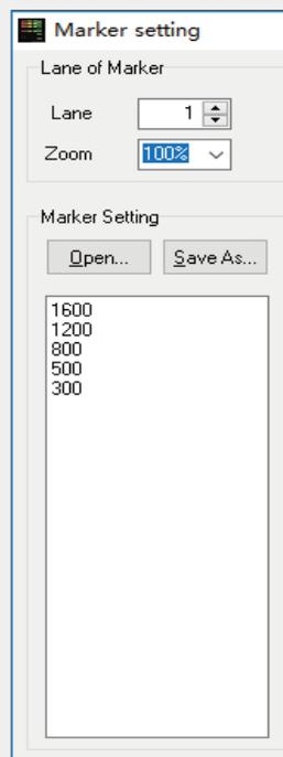
In the first time, you can input molecular weight base on the standard molecular weight , as shown on the left, we enter “1600, 1200, 800, 500 and 300” from top to bottom. You can save these configuration into the file as format “.cmr” by “Save As” button in order to use it in the next time without inputting the same molecular weight again.
