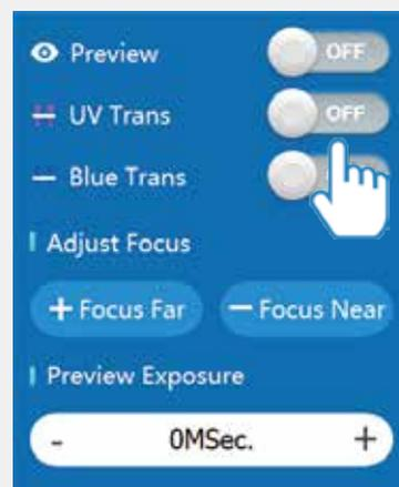
If you are using the ChemiScope 6000 Touch Series, you can turn on the UV transilluminator by touching the bar. (as shown on the left)
