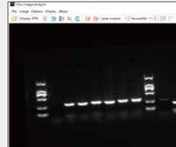
When the bands of the original image is not horizontal (as shown on the left). We can also use this function to put bands horizontally for image analysis.
