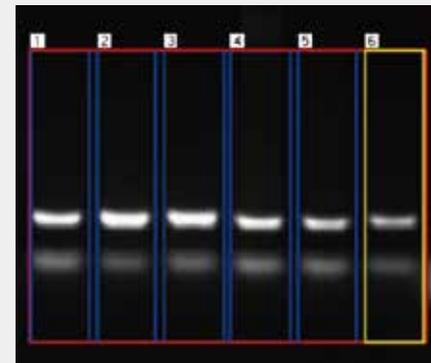
After setting, hold left mouse button to select the area you want to identify. It will be framed if the number of the bands is set to 6. The size and distance of each band is fixed.
