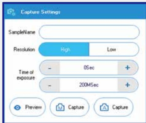
You enter sample name in the input box, the pictures will be automatically saved into the specified path after shooting every time.
