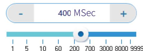
The longer exposure time is, the brighter picture is. The user can adjust exposure time according to different application. What You See Is What You Get when you adjust the exposure time under preview mode.
