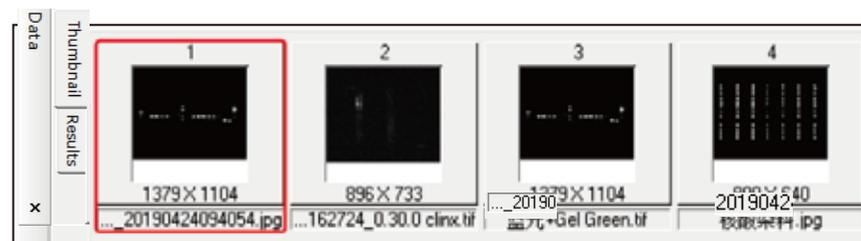
Once the band is recognized, the thumbnail window will automatically switch to the data window. You can also switch manually by clicking the "Thumbnail" or "Analysis Report" tab on the left.
