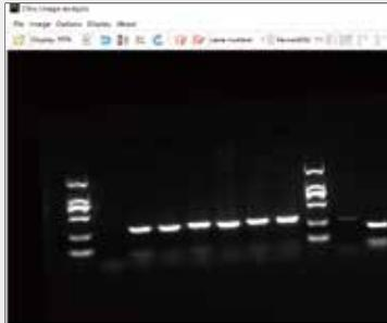
When the bands of the original image is not horizontal (as shown on the left). We can use this function to put bands horizontally for image analysis.
