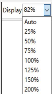
On the right side of the short-cut bar, you can adjust the size of the image in the main window by using the drop-down box, or you can select "Auto" function to automatically match the size of the image.
