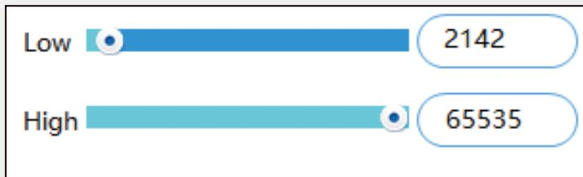
We firstly need to capture images before adjusting grayscale. To adjust grayscale range is for the background and the brightness of bands to be best to watch. The grayscale range is from 0 to 65535.
