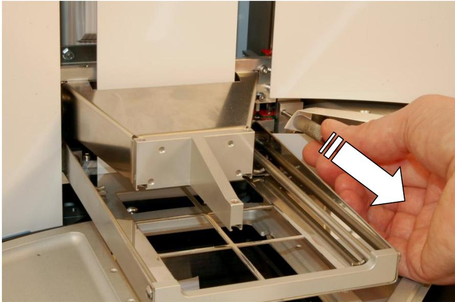
**Figure 4.** Tip comb holder transport lock removed
