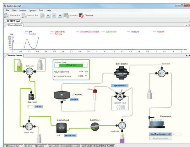
**Fig 9.** The **System Control** flow scheme represents the real-time flow path with indications of the different modules on the wet side of the instrument. The current run status of the system is displayed, together with the real-time chromatogram. The instrument can be controlled via clicks on the flow path, for example, to turn the valves, set flow rates, change buffer B concentrations, and start/stop fractionation.
