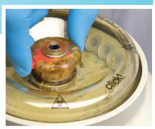
First in the industry, ClickSeal biocontainment lids provide certified, ergonomic, one click rotor opening and closing.
