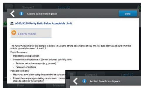
The A260/A280 ratio of sample #3 is outside the acceptable range for pure DNA. Learn about possible causes and review recommended solutions.
