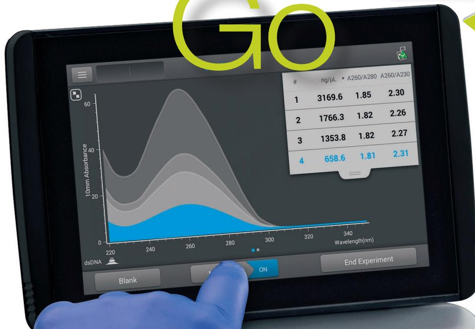
After blanking, load 1–2  $\mu\text{L}$  of your sample and lower the arm. Measurement results with full-spectral data will be displayed in seconds. Swipe left to view expanded data table.
