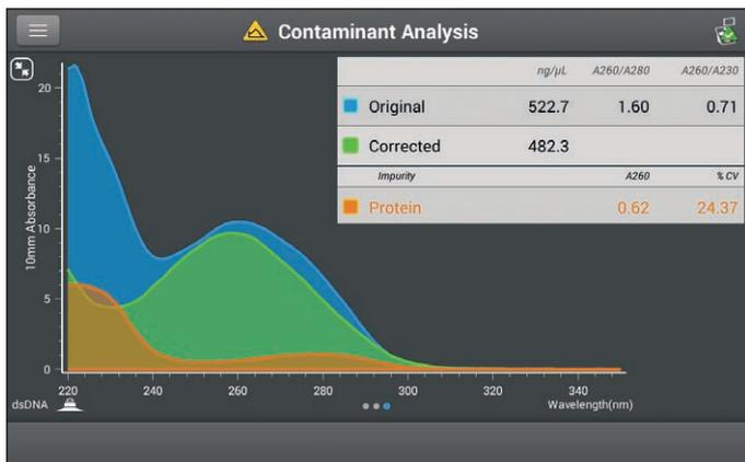
dsDNA sample contaminated with protein. The absorbance contribution from the protein (orange) is subtracted from the original result (blue) to obtain the corrected dsDNA concentration (green).
