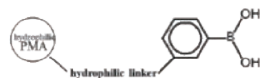
Figure 1. MC-Boronate affinity resin structure
