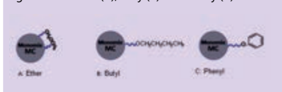
Figure 1 HIC Ether(A), Butyl(B) and Phenyl(C) Structure
