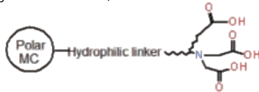
Figure 1b. Polar MC30/60-Ni Excel resin structure
